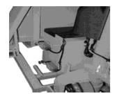
To lower the load further, select "Off" on the control box. After this, the load is lowered to the desired height using the manual lowering function on the towbar (see applicable section concerning this)
