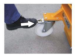
To release the parking brake press firmly against the lug.
