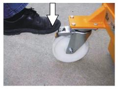
To activate the parking brake press firmly on the lug.
